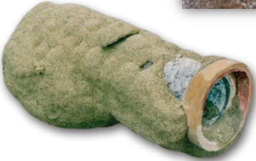
Tube-gel technology being used to seal private pipes
