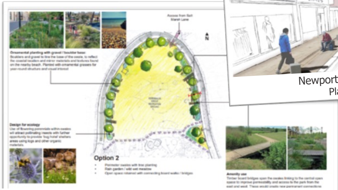
Cornwallis Circle, Whitstable Managing 1.2 hectares of impermeable area with regreening; featuring swales and tree planting
